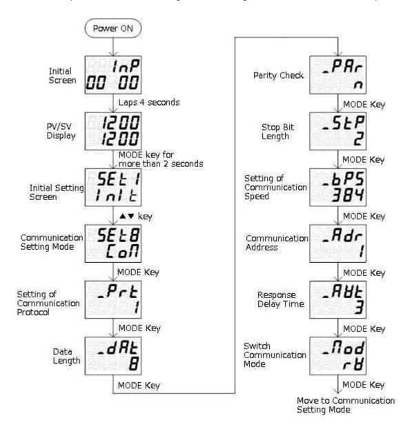
When the setting is done, press the MODE key for more than two seconds to return to operation mode. Communication setting mode is a setting mode that is common for channels. It can change the communication setting with the following operation regardless of the selection of CH:
